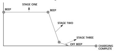
**Stage One** — Rapid Start Charge at 15 amps delivers maximum charging amperage to "wake up" any serviceable 12 volt battery and allows for quick engine starting in just  $3\frac{1}{2}$  minutes (based on a midsize vehicle battery at 50% charge level). When battery reaches a maximum safe predetermined voltage, the charger will automatically signal a "beep" and move into Stage 2 of the charging process.
